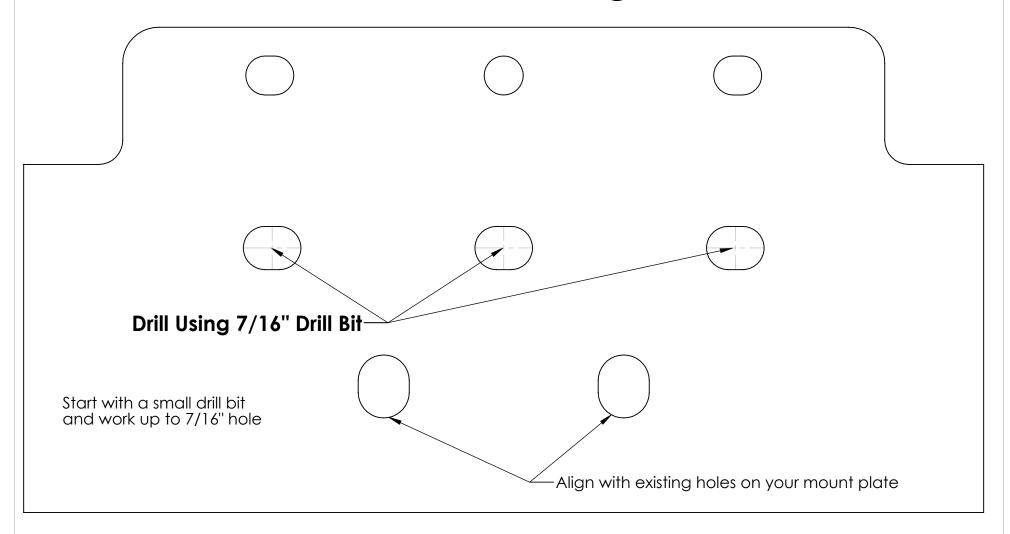
Check against the holes in your machine before drilling.
